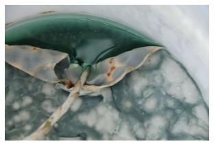
7. This delightful biofilm developed on the Dosatron feed bucket containing fertilizer and citric acid after sitting about a week, something that never happens if only fertilizer concentrate is in the bucket. A second Dosatron was ultimately added, one for the citric acid and one the fertilizer.
