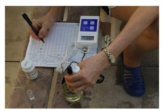
5. Keep careful records of the impact of citric acid addition rates. A Bluelab combo pH and conductivity meter was used to measure the pH of untreated and acidified water. The pH meter was used to verify proper acid addition rates with a target goal of 5.8 to 6.2.
