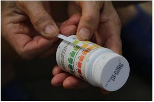
6. WaterWorks pH and total alkalinity test strips and Hach alkalinity test strips are reasonably accurate at the lower alkalinity levels to give you a general sense of the alkalinity of acidified water, but don't rely upon them to verify your target pH or alkalinity goals.
