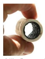
5. When Terry was replumbing the greenhouse water lines, he cut away an old section of pipe that containing a sticky, organic buildup on the inside of the PVC pipe. This deposit is a biofilm that develops inside irrigation lines, possibly exacerbated by the prior use of the pond behind the house for water.
